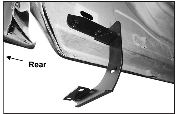
(Figure 18) Driver/left rear Bracket installed.
