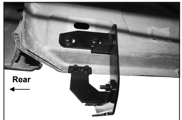
(Figure 20) Driver/left Rear Bracket assembly complete installation.
